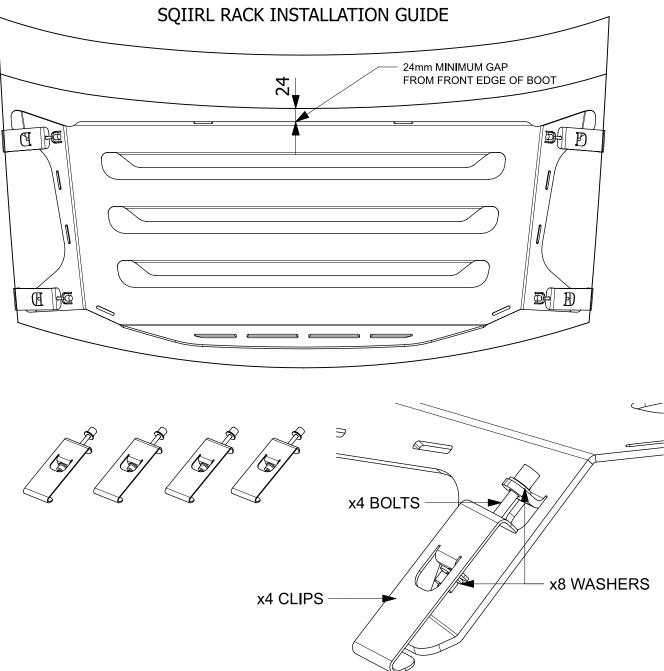
First prop the boot lid open to around 15 degrees and make sure it is not going to slam shut while you are positioning and securing rack.
